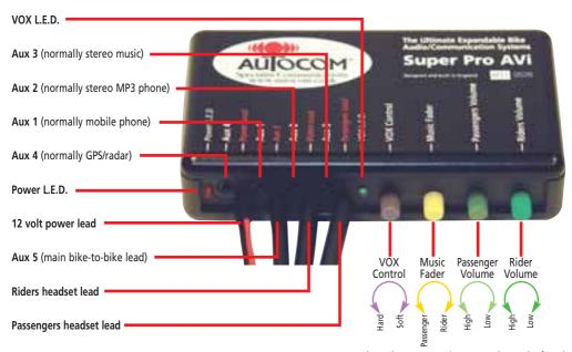
When the arrow pointers on the end of each control face towards the label it is set to the standard settings for used without earplugs, with music equal to both rider and passenger and automatic VOX on medium.
